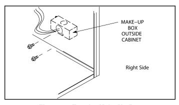
Figure 54. Exterior Make-Up Box (Field Provided Right Side)
