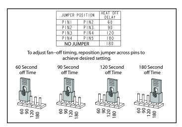
Figure 60. Heat Fan-OFF Time in Seconds
