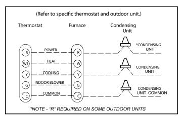
Figure 55. Furnace & Condensing Unit Thermostat Designations
