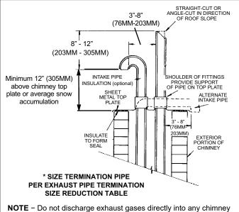
or vent stack. If vertical discharge through an existing unused chimney or stack is required, insert piping inside chimney until the pipe open end is above top of chimney and terminate as illustrated. In any exterior portion of chimney, the exhaust vent must be insulated.
