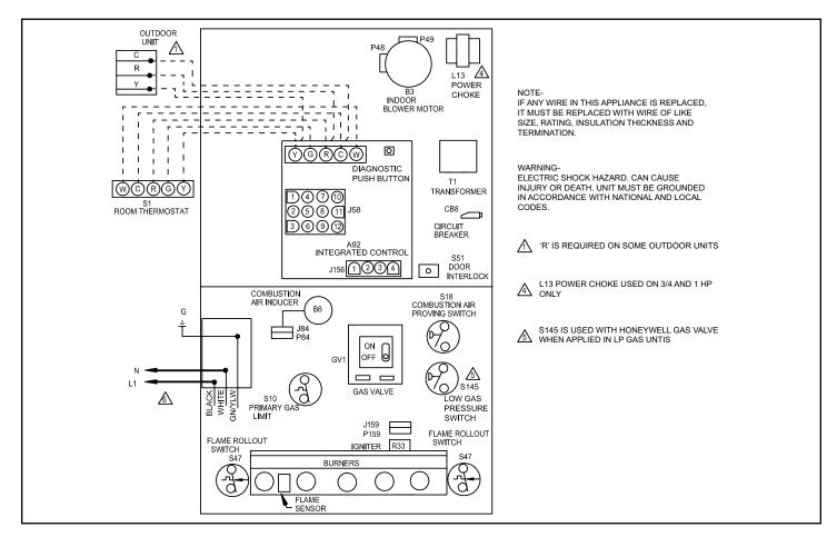
Figure 56. Typical Field Wiring Diagram
