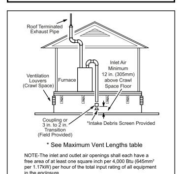
Figure 26. Equipment in Confined Space (Inlet Air from Ventilated Crawl Space and Outlet Air to Outside)
