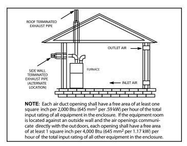
Figure 7. Equipment in Confined Space - all Air from Outside
