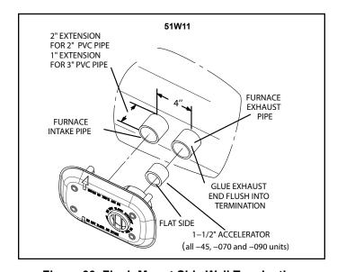
Figure 30. Flush Mount Side Wall Termination
