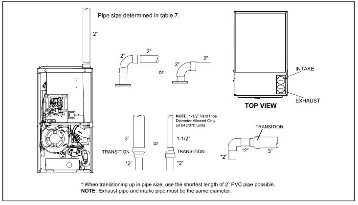
Figure 23. Typical Intake Pipe Connections (Direct Vent Applications)
