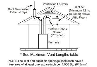
free area of at least one square inch per 4,000 Btu (645mm² per 1.17kW) per hour of the total input rating of all equipment in the enclosure.
