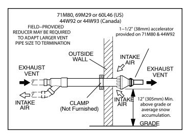
Figure 35. Direct Vent Concentric Wall Termination
