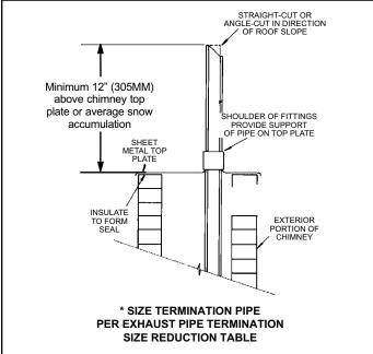
**NOTE** – Do not discharge exhaust gases directly into any chimney or vent stack. If vertical discharge through an existing unused chimney or stack is required, insert piping inside chimney until the pipe open end is above top of chimney and terminate as illustrated. In any exterior portion of chimney, the exhaust vent must be insulated.
