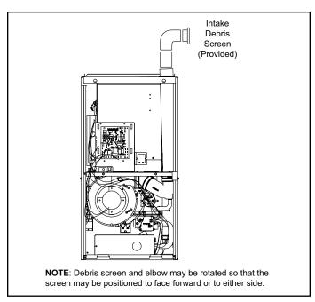
Figure 24. Typical Air Intake Pipe Connections
