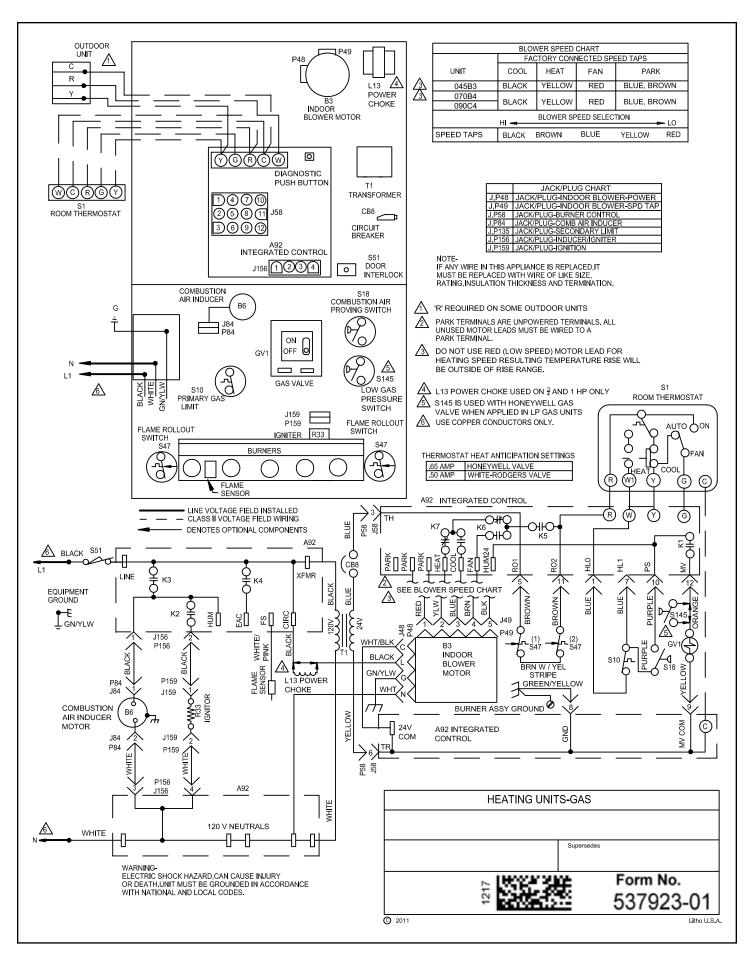
Figure 57. Typical Wiring Diagram
