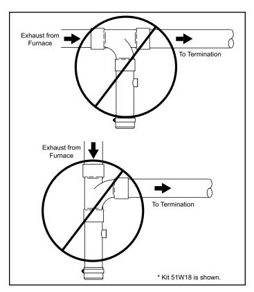
Figure 43. Crawl Space Vent Pipe Drain Trap
