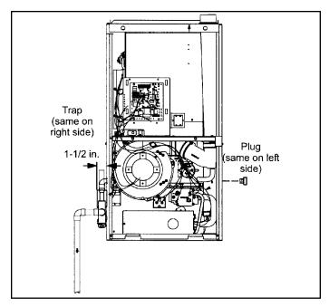
Figure 45. Condensate Trap and Plug Locations
