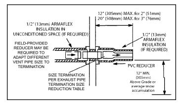
Figure 39. Non-Direct Vent Field Supplied Wall Termination
