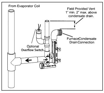
Figure 49. Condensate Trap with Optional Overflow Switch
