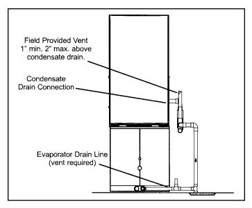
Figure 48. Evaporator Coil Using a Common Drain
