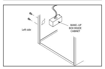
Figure 53. Interior Make-Up Box (Factory - Installed Left Side)
