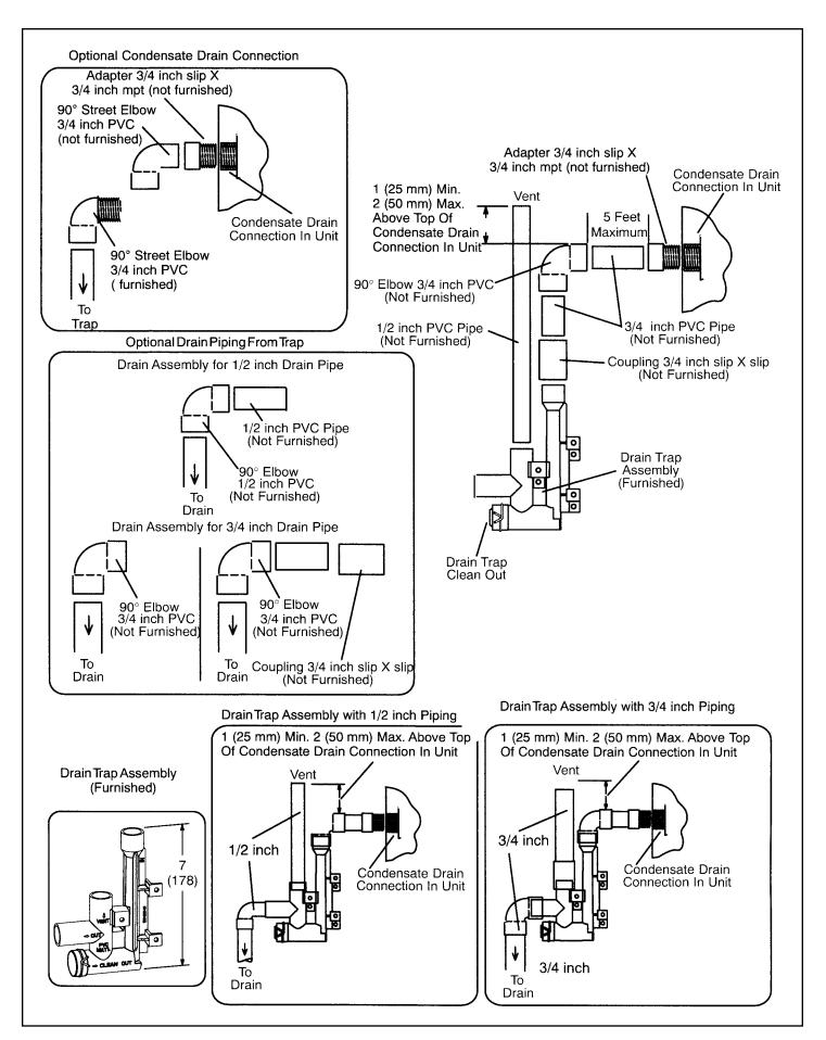
Figure 50. Trap Drain Assembly Using 1/2" PVC or 3/4" PVC
