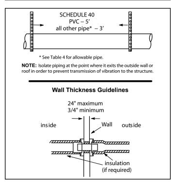
Figure 19. Piping Suspension Guidelines
