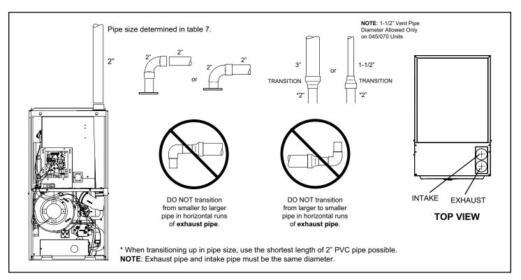
Figure 22. Typical Exhaust Pipe Connections
