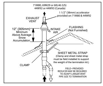
Figure 37. Direct Vent Concentric Rooftop
