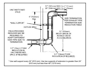
Figure 40. Non-Direct Vent Field Supplied Wall Termination Extended
